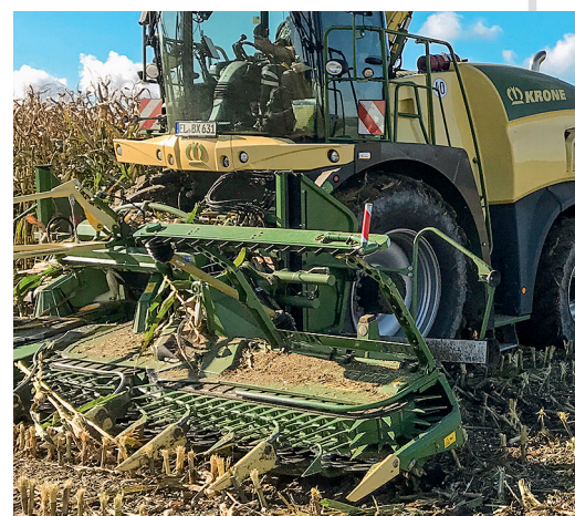
In our testers' opinion, the active feed system is better in tall maize than the hoop.
