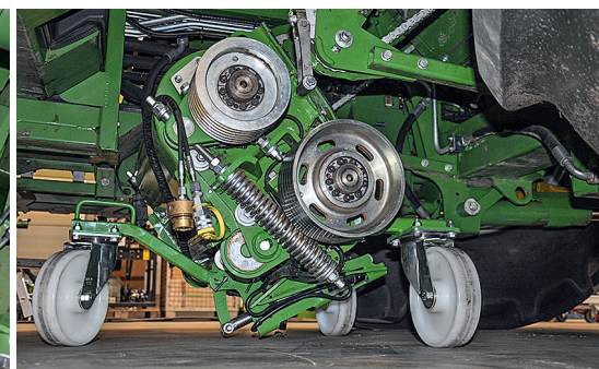
'VariQuick' allows quick changeovers between maize and grass or wholecrop. The corn cracker is lowered on a chain and pulled out to the side on rollers.
