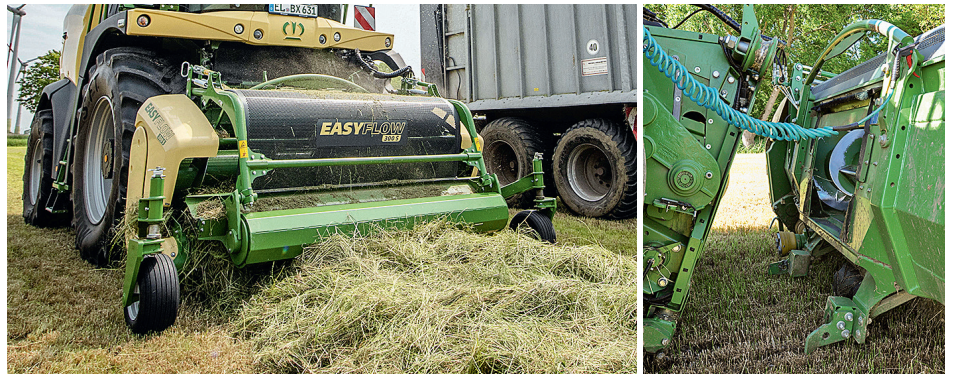
The EasyFlow 300S pick-up showed no real design weaknesses when on test ... except for the friction clutch for the auger. Right: The header and harvester can move apart slightly with the hoses still connected when giving the area a thorough blow-down with a compressor.
