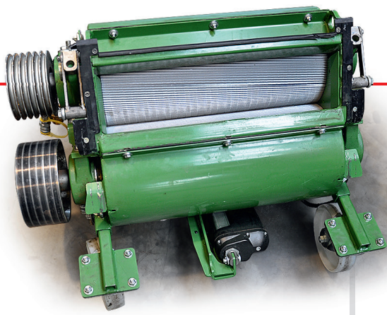
The 'BusaClad' hard-wearing surface coating is intended to extend the service life. It costs a significant £15,365 so takes some justifying.
