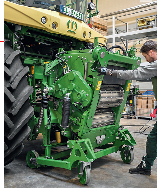
A service trolley is available for both the intake unit and the drum to make changes easier.
