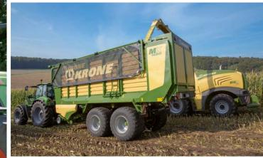
MX, this is the designation for high-performance large-capacity loading and forage transport wagons with a transport volume of 33 m<sup>3</sup> to 40 m<sup>3</sup>. Genuine dual-purpose forage wagons, they run in both the grass harvest chain as self-loading machines with discharge rollers and in the maize transport chain as forager-filled silage trailers. These machines score on versatility, reliability, efficiency and flexibility.
