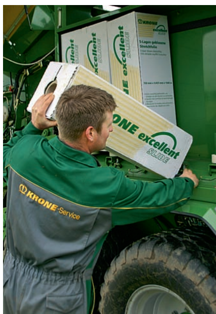
There is room on the CF155 to accommodate up to ten spare rolls of wrap via this neat hinged storage.
