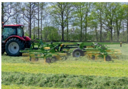
Four-rotor centre delivery rakes Swadro TC 1250 Variable, 9.80 m to 12.50 m work widths
