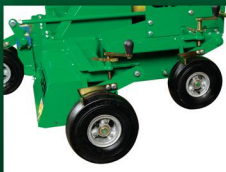
Wheescrapers stop build up of cut matter on wheels.
