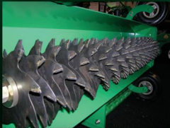
A bottom view of the GBS 200 shows its standard 39 blade setup.
