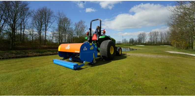
Compaction is a problem for groundsman and greenkeepers worldwide. Aeration of compacted sports fields and golf courses is a common practice in all renovations and maintenance programs. The GKB Deep Tine Aerator can penetrate through the compacted turf with various tine sizes on different depths. Surface water can pass through the profile and it allows air into the root structure which leads towards a healthier grass plant and improved surface.
