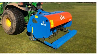
With an adjustable 25-degree heave angle, the Deep Tine Aerator's tine holding system allows you to take control on removing compaction from various depths up to 40 cm.
