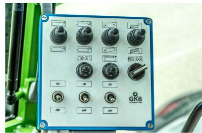
GKB offers various systems for adjusting the sand distribution. A mounted or movable adjustment system are one of these options. In addition to the hydraulic-electric proportional control, the sand gate is also hydraulically adjustable.
