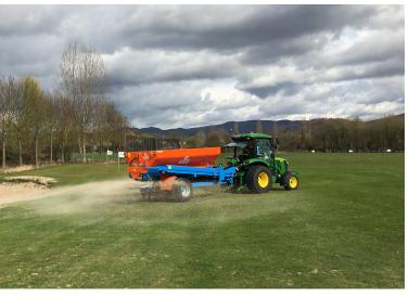
In addition to the SP model, there is also the SPM model. Beside the characteristics of the SP model, the SPM model has a conveyor belt. What gives you the opportunitie to top up the sand bunkers on golf courses. Because with the SPM model you are able to fill sand bunks.
