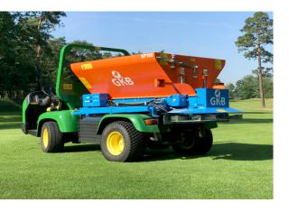
The Sandspreader is available in four distinctive designs. The capacity of the bunker varies from 1 m<sup>3</sup> to 4 m<sup>3</sup>. The Sp100 is suitable for assembling on a turf truck. For instance, on a ProGator, Truckster or Workman.
