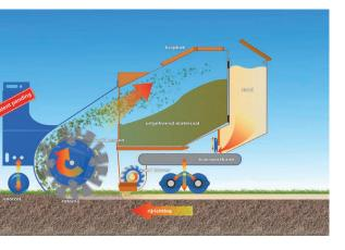
As the foundation of the Sandfiller we are making use of the clarified principle of the much-praised Combinator. The slitting rotor is provided with an attachment to the carbide blades that create wind to move the material to the sidewaystipping container. After you have emptied the sideways-tipping container, you can simply refill the container with dried sand.
