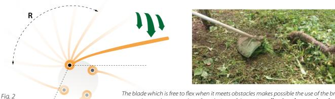
The blade which is free to flex when it meets obstacles makes possible the use of the brush cutter also to a lower number of revolutions of the engine, **allowing the use also close to** the plants without damaging the stem.
